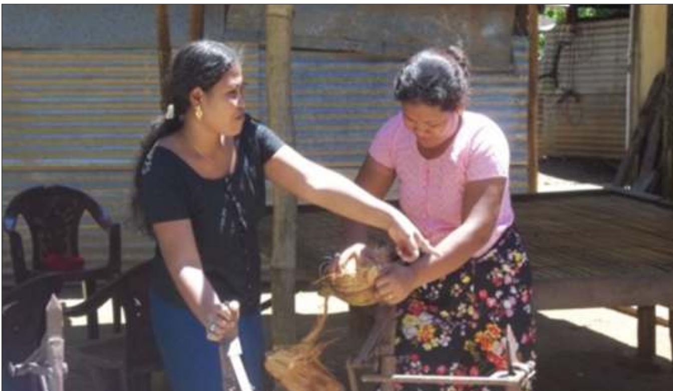
Coconut dehusker to reduce drudgery at Carnicobar (A&N Islands)
